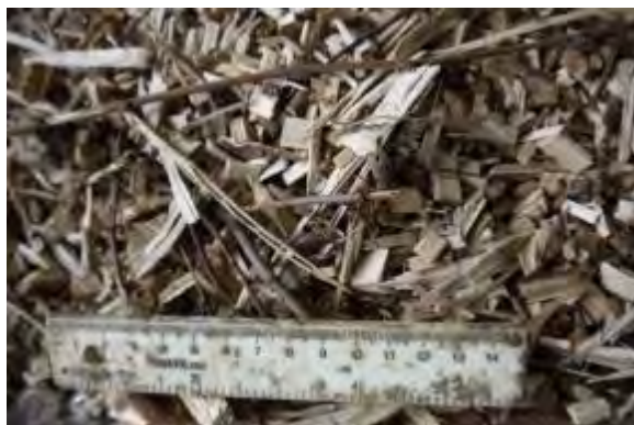
Figure 4.6. Hedgerow woodchip produced by the Timberwolf TW 150 DHB disc chipper
