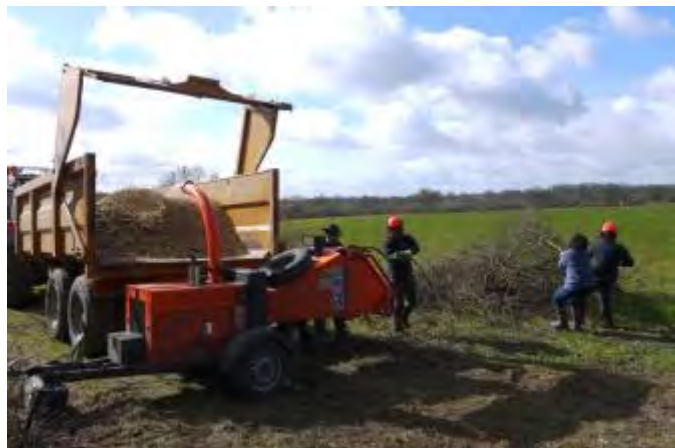
Figure 4.5. Extracting and hand feeding hedgerow material into the Timberwolf disc chipper at Elm Farm
