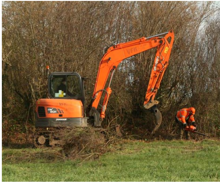
Figure 3.9. The assisted fell technique: chainsaw plus excavator mounted land rake coppicing Hedge 21 Elm Farm
