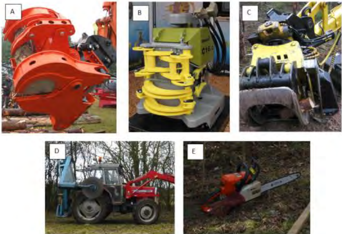
Figure 2.1. Different types of timber harvesting machinery: A) hydraulic shears, B) integral circular saw, C) integral chainsaw cutting bar, D) circular saw, E) chainsaw.
