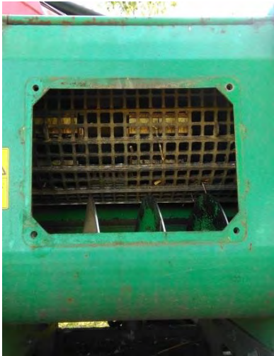
Integral 35mm woodchip screen in the Jenz HM360 chipper, also found in the Heizohack chipper
