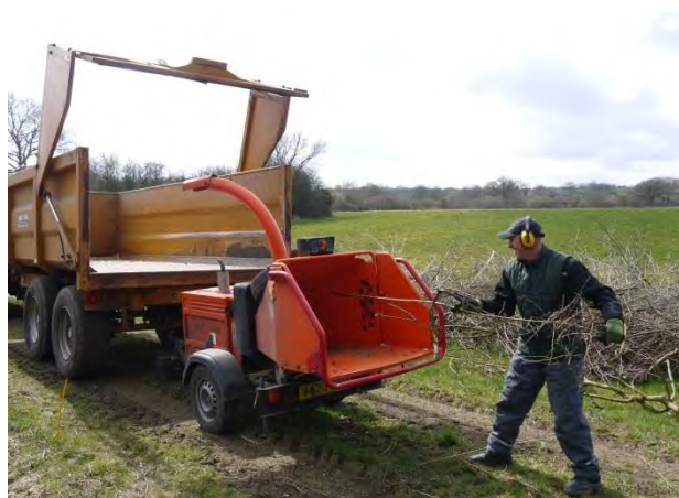
Figure 3.123. The diesel powered 6" Timberwolf disc chipper being used to chip material from Hedge 21 at Elm Farm
