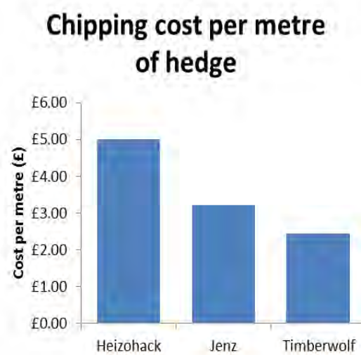
Figure 5.10. Chipping cost per metre of hedge for the chippers trialled. Costs are based on each machine being used at their maximum efficiency per day
