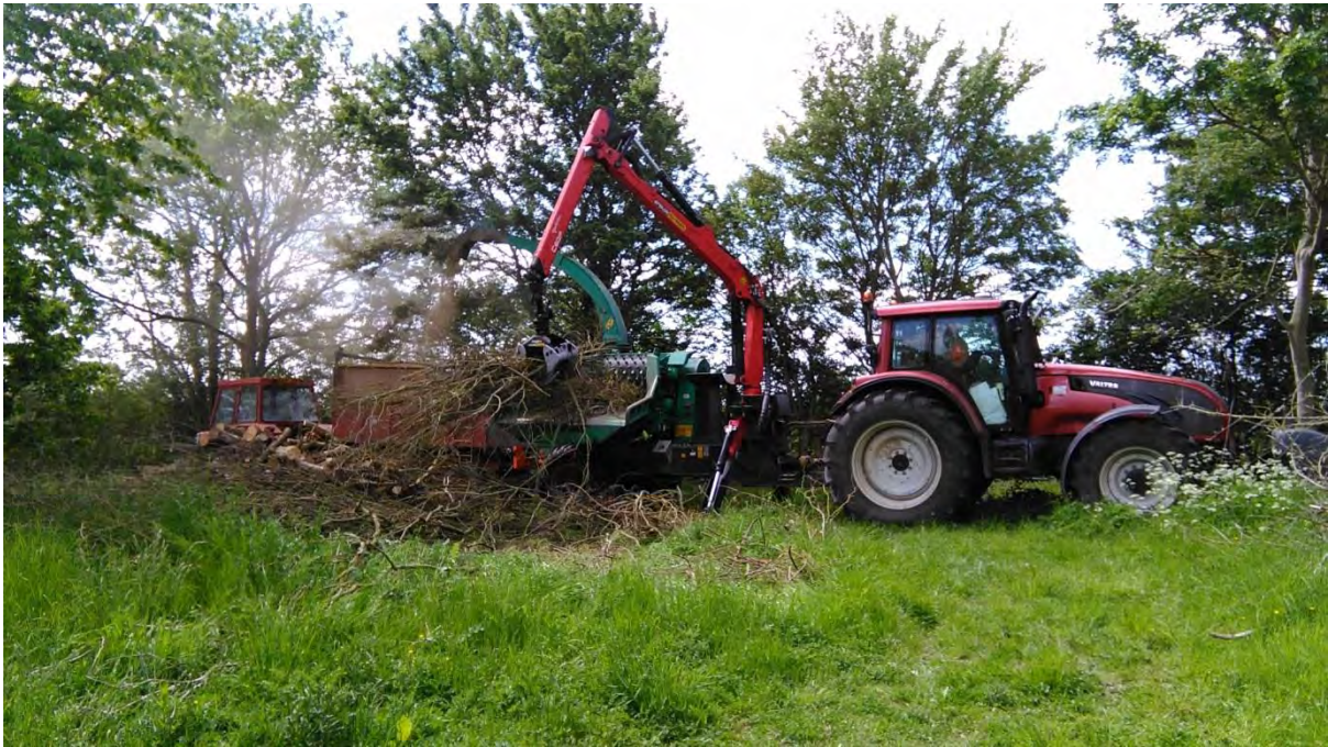
Figure 3.12. The tractor towed Jenz HM360 fuel grade drum chipper with 8.6m telescopic crane chipping material from Hedge 1 at Wakelyns Agroforestry.
