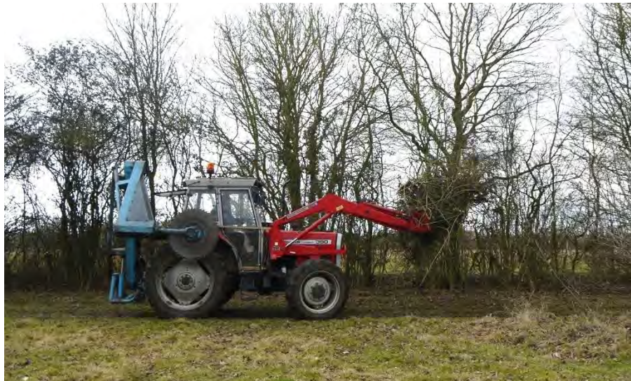
Figure 3.8. The circular saw: A 36"/900mm mechanically-driven single blade Fisher Humphries circular saw, mounted on a Massey Ferguson 390 tractor with a front-mounted fork moving hedgerow material after coppicing Hedge 1 at Wakelyns Agroforestry
