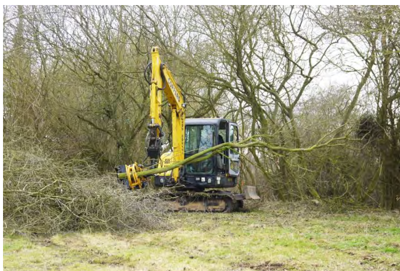
Figure 3.7. The felling grapple with integral chainsaw cutting bar: Excavator mounted Gierkink GMT 035 felling grapple, coppicing Hedge 1 at Wakelyns Agroforestry
